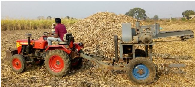
Figure 10 Tractor operated biomass shredder
